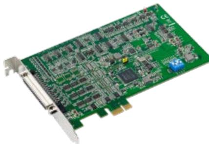
DAQ Card and distribution panel (DISPAN) are in connection by SCSI cable. DISPAN and DAQ card has female SCSI connectors. It comes with SCSI cable connected.
